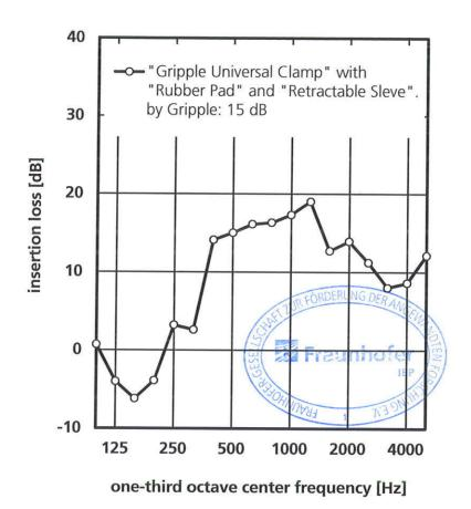
Frequency response of the insertion loss by noise excitation by a standardized source of installation noise (IGN), measured in the test room EG front (vertical, installation room UG front). The A-weighted sound level reduction  $\Delta L_{A,F}$  in dB (referring to IGN noise excitation), for the reproduced frequency range from 100 to 5000 Hz, is represented in the legend.
