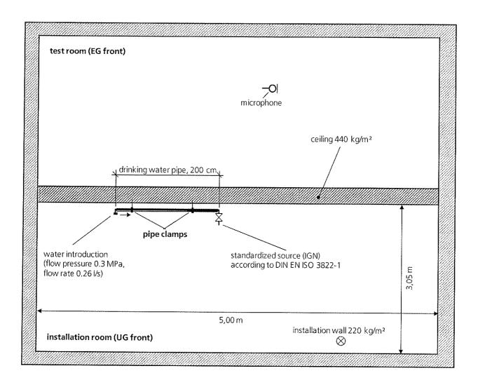
Test set-up for the determination of the insertion loss of structure-born insulating tubes or elastic mounting elements for drinking water pipes mounted on the ceiling (not to scale).
